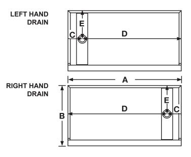
\* Make sure the drain hole in the subfloor or slab is large enough (6" diameter recommended) and aligns with the hole in the shower floor.
